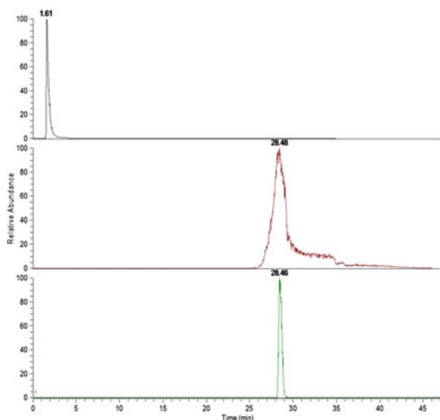
**Figure 1.** Comparison of the chromatography of ADP using C18, ZIC-HILIC and AS19 ion chromatography stationary phases. ADP elutes without being retained on the C18 column, ran with poor peak shape (FWHM peak width of 90 s) on the HILIC column, and produced a clear Gaussian peak with a FWHM peak width of 30 s under ion chromatography conditions.
