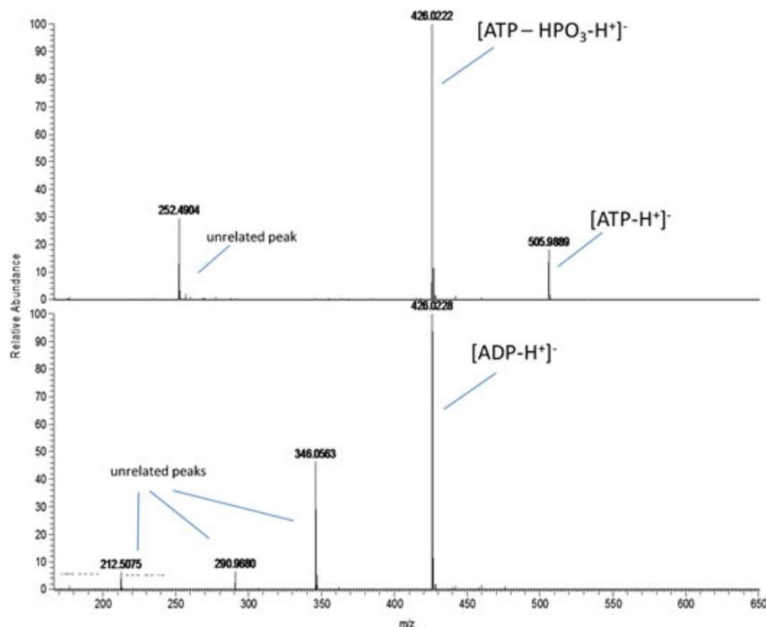
**Figure 2.** Spectra of ATP (top) and ADP (bottom). The peak at 505.9889 corresponds to the true mass of ATP. Loss of a phosphate group in source results in the dominant peak in the mass spectrum corresponding to ADP (426.0226).
