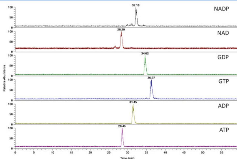
**Figure 3.** Separation of a group of compounds with poor retention on HILIC. These compounds are well retained using capillary flow ion chromatography and produce Gaussian peaks.
